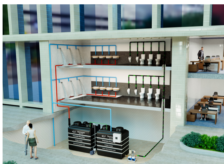
Image of a greywater recycling system in a commercial office space.
