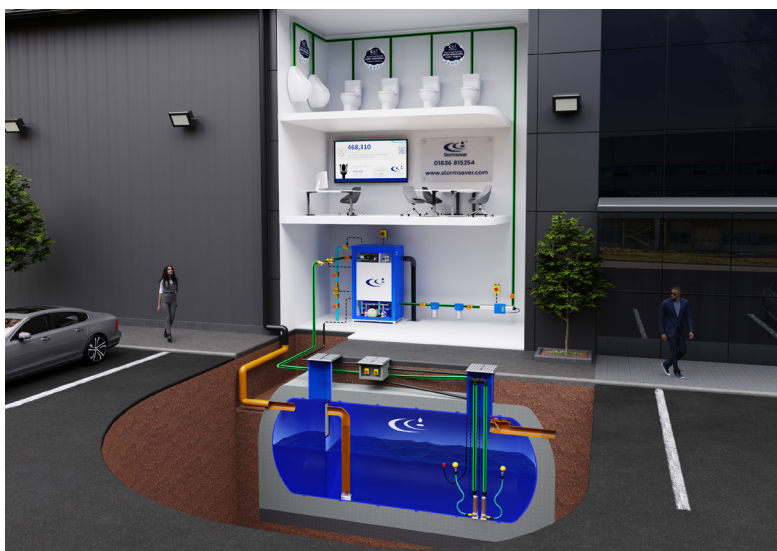
Image of a Combi style rainwater harvesting system in a non-household development.
